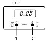
4. Within 5 seconds press and hold either button (1) to decrease or button (2) to increase the time until the correct time of day on the 24 hour clock is reached, e.g.14.30.
